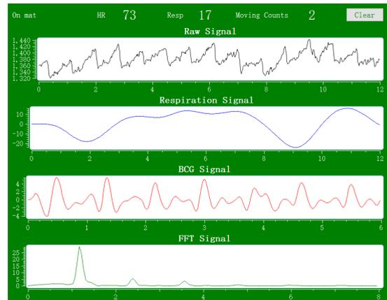
FIGURE 7: Real-time monitoring results with handheld module
