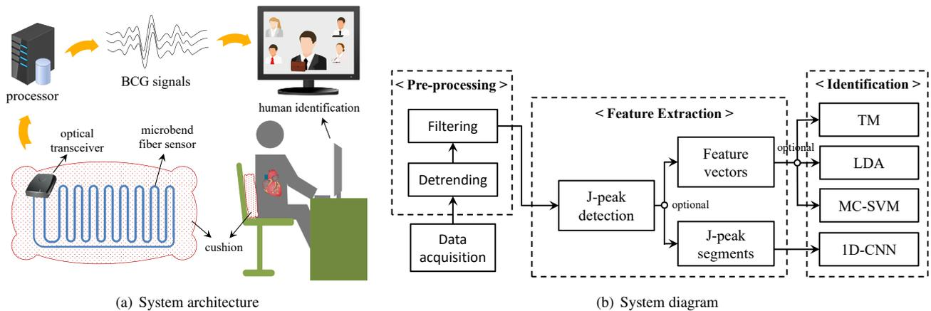
FIGURE 1: Proposed continuous human identification system
