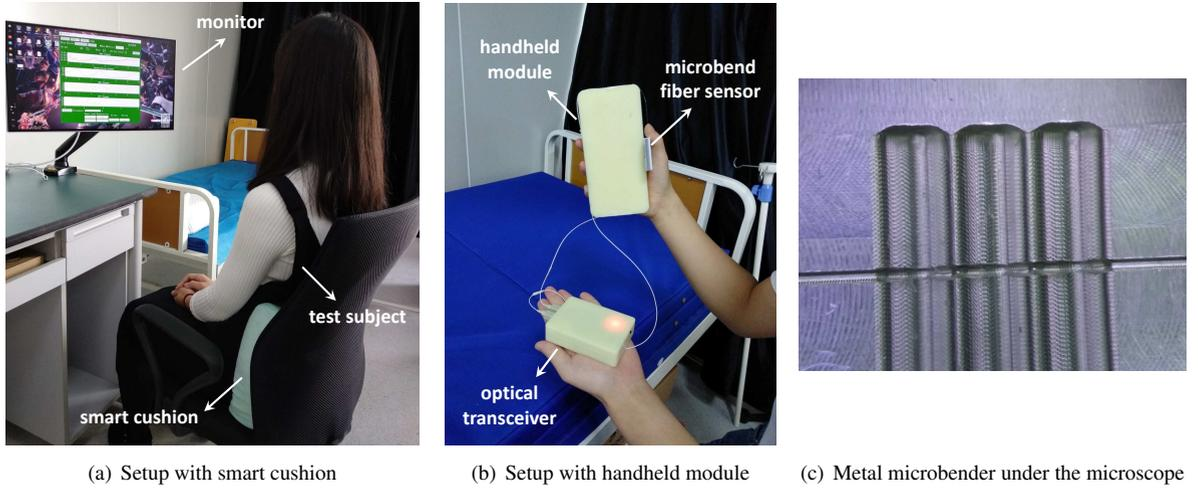
FIGURE 5: Experimental setup of the human identification system using a microbend fiber sensor
