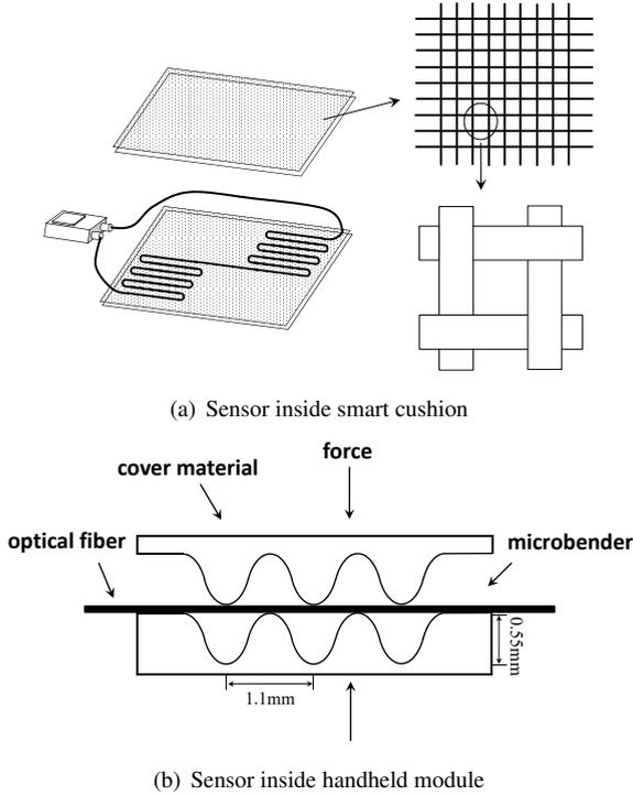
FIGURE 2: Schematic of the microbend fiber sensor
