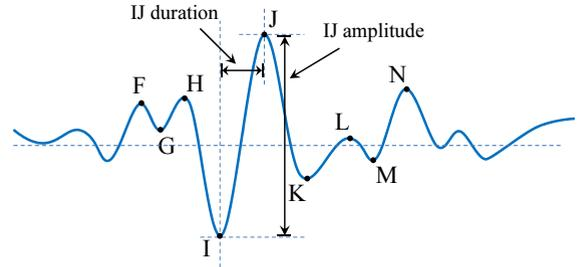
FIGURE 3: A typical BCG waveform of the normal human subject
